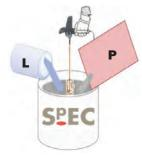
The liquid should be poured into a 25 litre plastic or metal drum. The powder should be added slowly whilst mixing with a spiral paddle attachment on a slow speed electric drill. Mixing should continue
